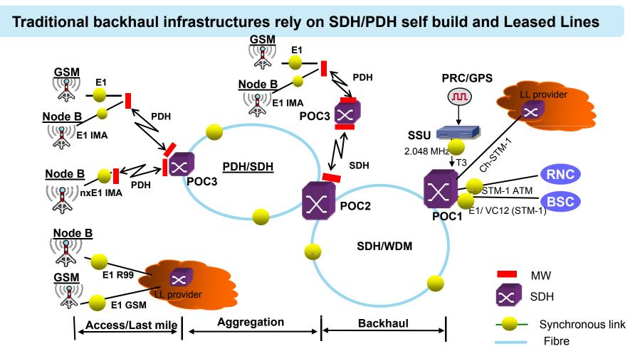
Ethernet migration critical to mitigate cost penalty given by ever increasing capacity requirements for packet-switched traffic (fixed and mobile broadband)
