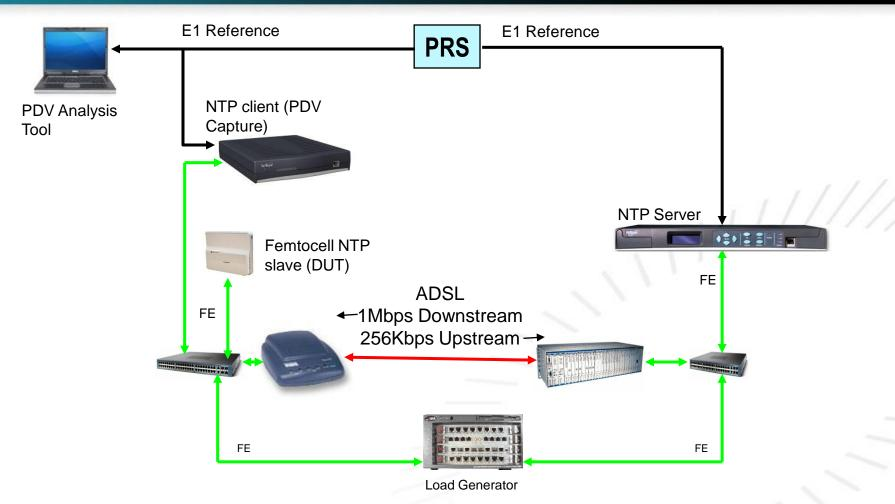
Maintain Femtocell Frequency (and Phase) accuracy in Asymmetric DSL
