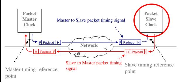
PEC: Packet based Equipment Clock PEC-S From G.8263 draft Local reference Time Scale Comparator **Packet Timing** Output Clock **Packet** Low Pass filter Oscillator Signal Selection Packet Selection 2 Local Time is key factor scale
