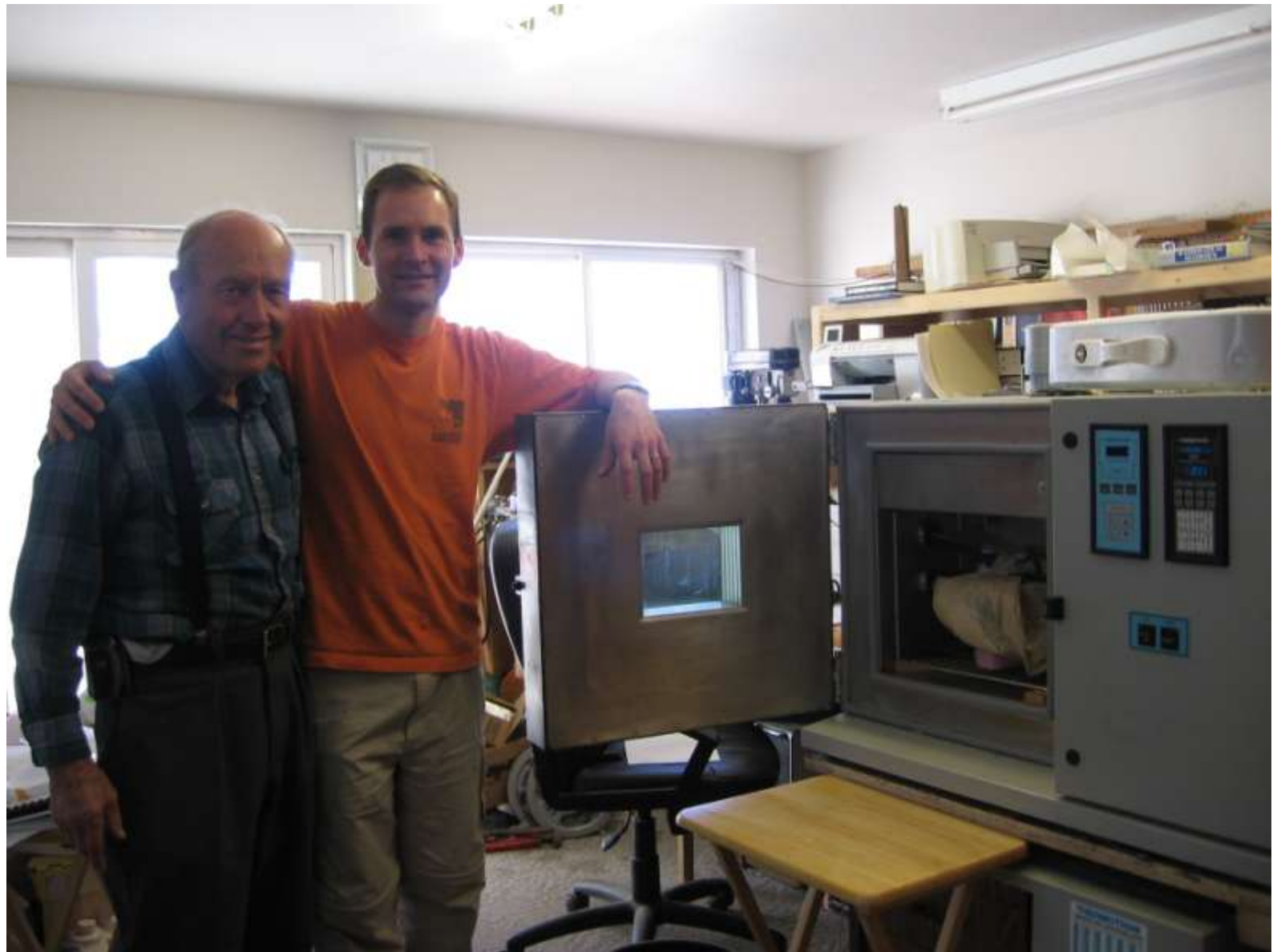
OVEN to test temperature independence of EQUATE timing package
