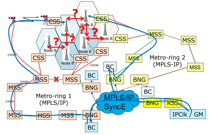
Requirements for adjacent clusters using different parts of the transport network providing timing for LTE-A with or without CoMP (coordinated multipoint)
