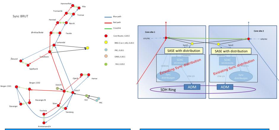
SyncE distribution in Telenor MPLS and IP/VPN CORE network Sync distribution from IP Core Network to SDH regional network
