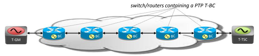
every switch/router on the path between T-GM and the T-TSC contains a T-BC
