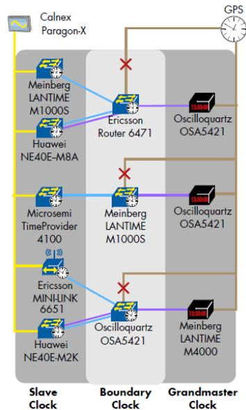
Time/Phase Holdover with Sync-E Support in the Core
