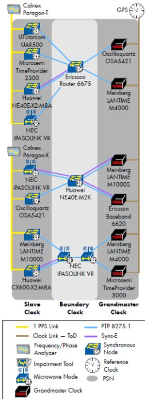
Grandmasters were provided with GPS signal from a common GPS antenna
