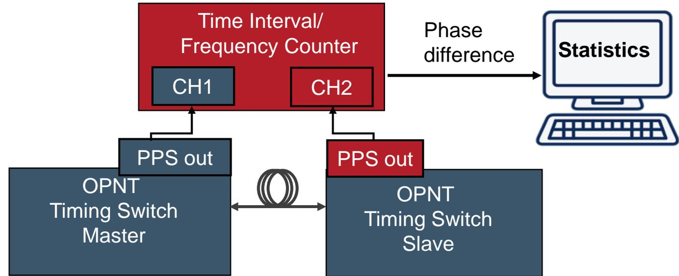
The pulse-per-second (PPS) output of the Master Timing Switch and the Slave Timing Switch are directly compared with each other using a Time Interval/Frequency counter.
