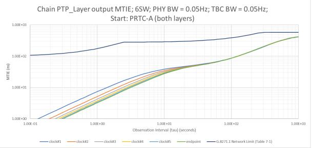
Expected MTIE of clock chain (PTP\_layer) (including endpoint) using oscillator with assumed performance (TDEV(@1s) = 0.1ns) for phy\_layer bandwidth of 0.05Hz and PTP\_layer bandwidth of 0.05Hz
