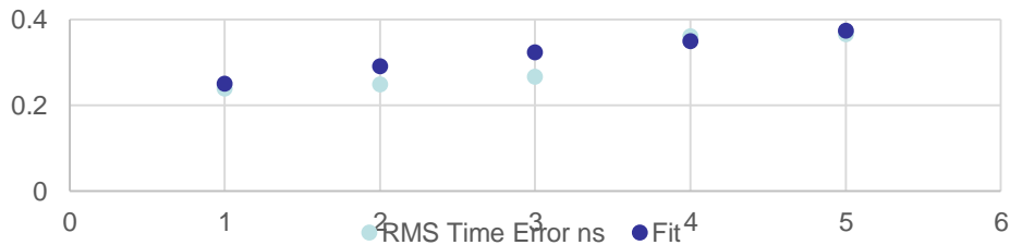
Peak Tdev Noise Accumulation Fit: 100 \text{ ps} + 150 \text{ ps} \cdot \sqrt{N}
