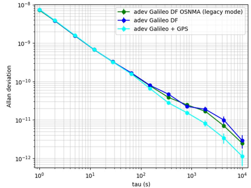
Allan deviation at the output of internal receiver
